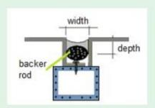
Install backing material, spacer, or joint filler to ensure correct depth to width ratio is achieved according to design. Apply masking tapes to areas adjacent to joints to ensure neat sealant lines.
